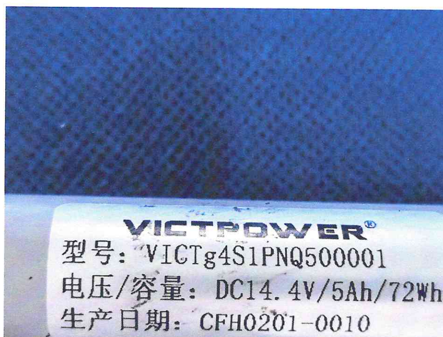
电池组铭牌 View of the battery nameplate
