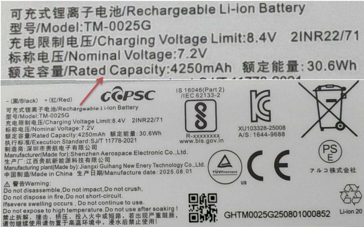
电池组铭牌 View of the battery nameplate
