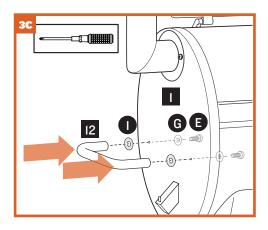
ATTACH HANDLE AND PLACE HEAT BAFFLE AND DRIP TRAY
